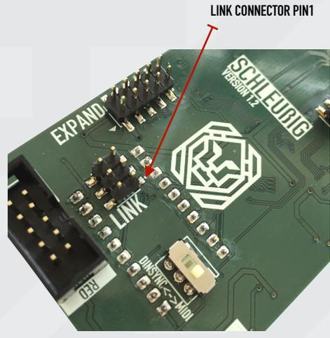
We also plan a footswitch expander that can be attached to the LINK connector.
