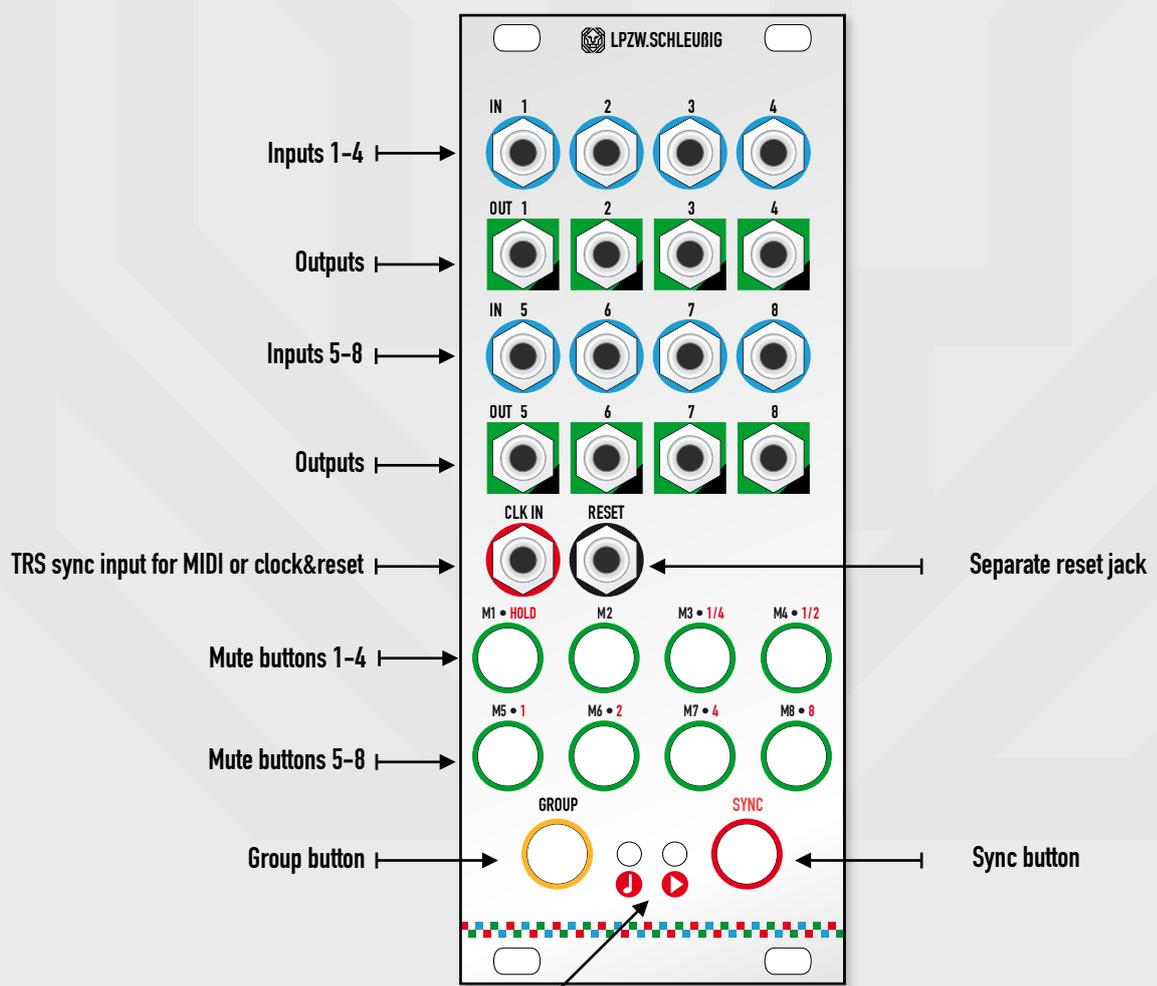
Timing indicator LEDs (1/4 note and sync point)
