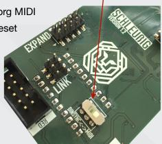
The **RESET** signal can be either a pulse or a permanent high level
