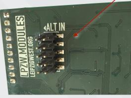
The expander is actually just an assembly of 8 jacks with no other electronics. All the circuitry for this function is already included on the main module, so you can build your own ALT IN expander. The pinout is:
