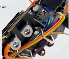
**Step 13:** connect the PO+adapter to your Eurorack. Make sure you align the red line with the marking on the adapter and the bus boards -12V!
