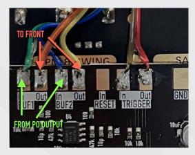
**Step 11:** The PO only recognises the rising edge of the clock, but there is no start/stop signal for synchronisation. So we need an additional signal from the "play" button, to reset the state of the clock signal.
